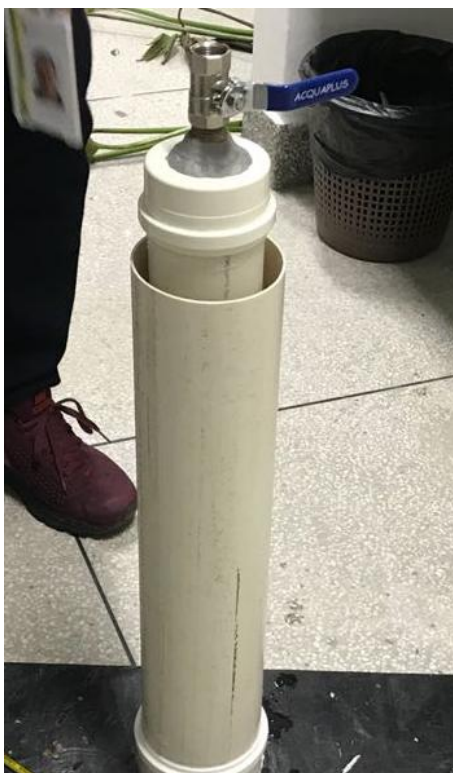
Figure 4. PVC biodigester used in the biogas production process. Source: Personal Collection, 2018.
