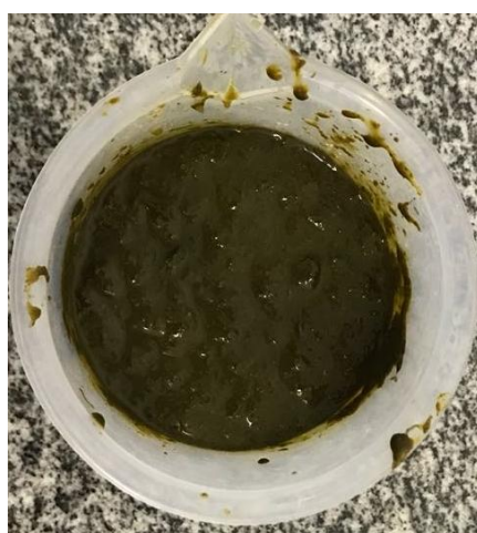
Figure 2. Mixture obtained from mashed Baronesa and bovine manure. Source: Personal Collection, 2018.
