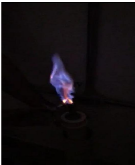
Figure 6. Flame test in the biodigester. Source: Personal Collection, 2018.
